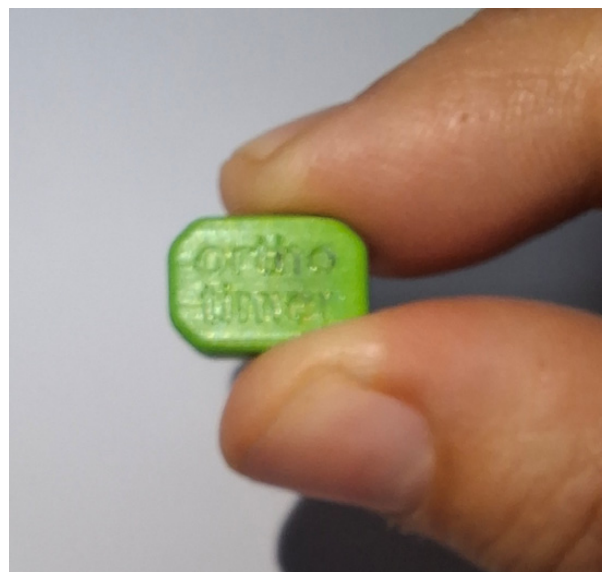
Figure 1. OrthoTimer ® thermal sensor positioned inside the brace.
